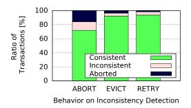
Fig. 6. The efficacy of T-Cache as a function of the strategy taken for handling detected inconsistencies. ABORT detects 55% of the uncommitable transactions, and EVICT and RETRY reduce the rate of uncommitable transactions to about 25%.
