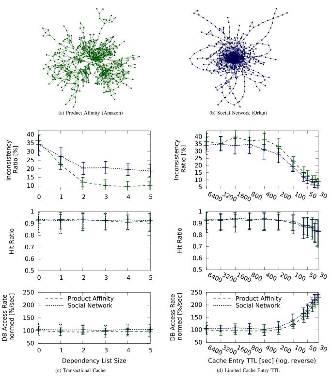
Fig. 7. Experiments with workloads based on a web retailer product affinity topology and a social network topology illustrated in (a) and (b). Transactional cache (c) compared against the alternative of reducing cache entry time-to-live (d). Data points are medians and error bars bound the 10 and 90 percentiles.
